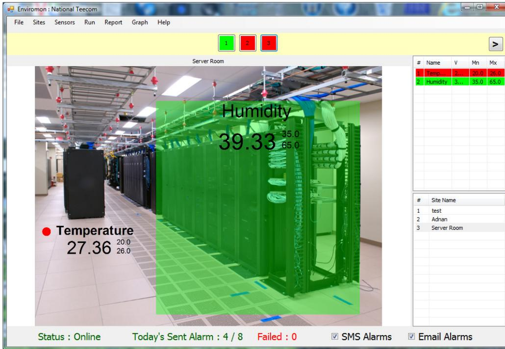
So on the image, sensors values are shown along with the ranges set for each sensor, the green highlight is for indicating that sensor reading is still within range, if not, the highlight will become red, user will be notified immediately whenever a parameter is out of range by E-mail and SMS message Example: Temperature at "site name you enter for site information normally your company name" the site name you named above which in on this example is Data center 27C° max is 26 C°
